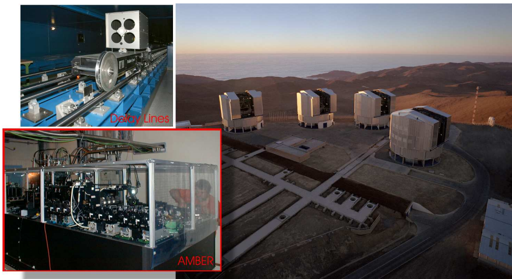
Figure 4.1: Mosaic of the VLT/VLTI infrastructure (4 UTs, to the right) with the AMBER instrument, which is located in the optical laboratory. In the upper left corner, one of reflectors of the VLTI delay lines is shown (Image Credits: ESO & AMBER consortium).
