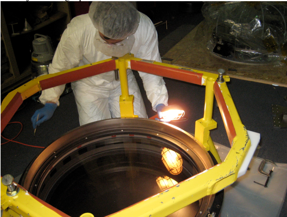
Joe Zajac cleaning optical surface with small brush.
