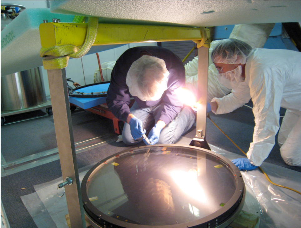
Joe Zajac cleaning optical surface with small brush.
