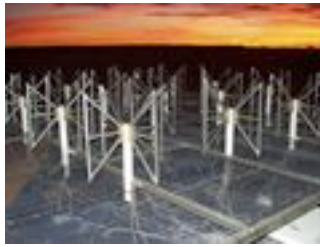
EAVESDROP Single antenna tile from the Mileura Wide-Field Array. Image
