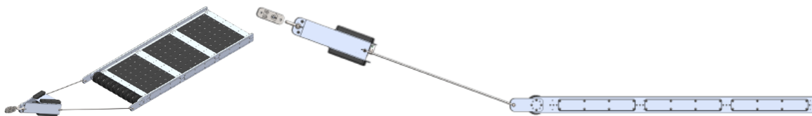
Figure 1: Magnetic sled design. Left: Isometric view of the magnetic sled design, Right: Side view of the sled when placed on the ocean floor. The 250-kg, 1 by 2 meter sled was covered with an array of 300 neodymium magnets on both sides and equipped with video cameras in the metal tow-halter ahead of it, which was anchored by a synthetic cable to a winch on the ship, the M/V Silver Star.
