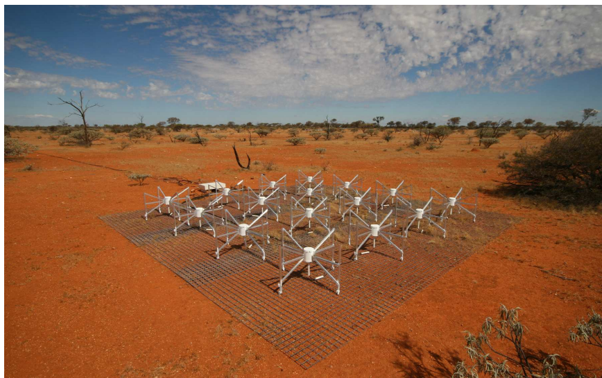
Figure 12.19 One of the antenna “tiles” used in the Murchison Widefield Array (MWA) experiment in Western Australia (see Color Plate 30 for a color version of this figure). Each such tile is composed of 16 crossed-dipole antennae, with their signals combined through hardware at the station. The full telescope combines the signals from \sim 128 tiles interferometrically. This allows for a large (several hundred square degree) field of view with a moderately large collecting area. The antennae operate between 80–300 MHz, corresponding to z \approx 6 –15 (although the telescope will only be sensitive to the spin-flip background at z < 10 ). Image credit: C. Lonsdale.
