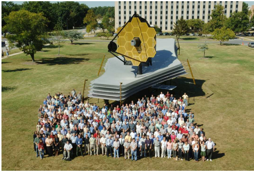
Figure 10.2 A full scale model of the James Webb Space Telescope (JWST), the successor to the Hubble Space Telescope ( http://www.jwst.nasa.gov/ ; see Color Plate 19 for a color version of this image)). JWST includes a primary mirror 6.5 meters in diameter, and offers instrument sensitivity across the infrared wavelength range of 0.6–28 \mu\text{m} which will allow detection of the first generations of galaxies. The size of the Sun shield (the large flat screen in the image) is 22 meters \times 10 meters (72 ft \times 29 ft). The telescope will orbit 1.5 million kilometers from Earth at the Lagrange L2 point. Figure credit: NASA/EPO.
