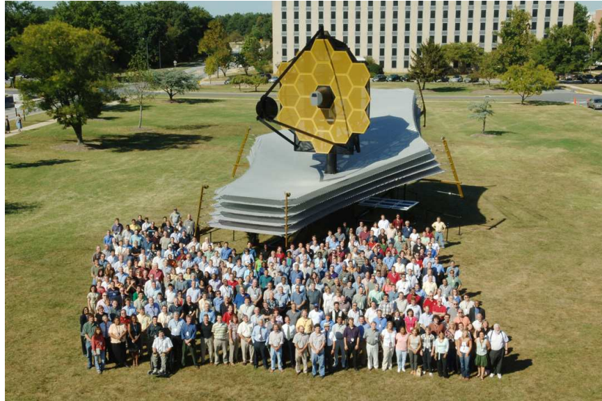
Figure 12.6 A full scale model of the James Webb Space Telescope (JWST), the successor to the Hubble Space Telescope ( http://www.jwst.nasa.gov/ ). JWST includes a primary mirror 6.5 meters in diameter, and offers instrument sensitivity across the infrared wavelength range of 0.6\text{--}28\mu\text{m} which will allow detection of the first galaxies. The size of the Sun shield (the large flat screen in the image) is 22 meters \times 10 meters (72 ft \times 29 ft). The telescope will orbit 1.5 million kilometers from Earth at the Lagrange L2 point.
