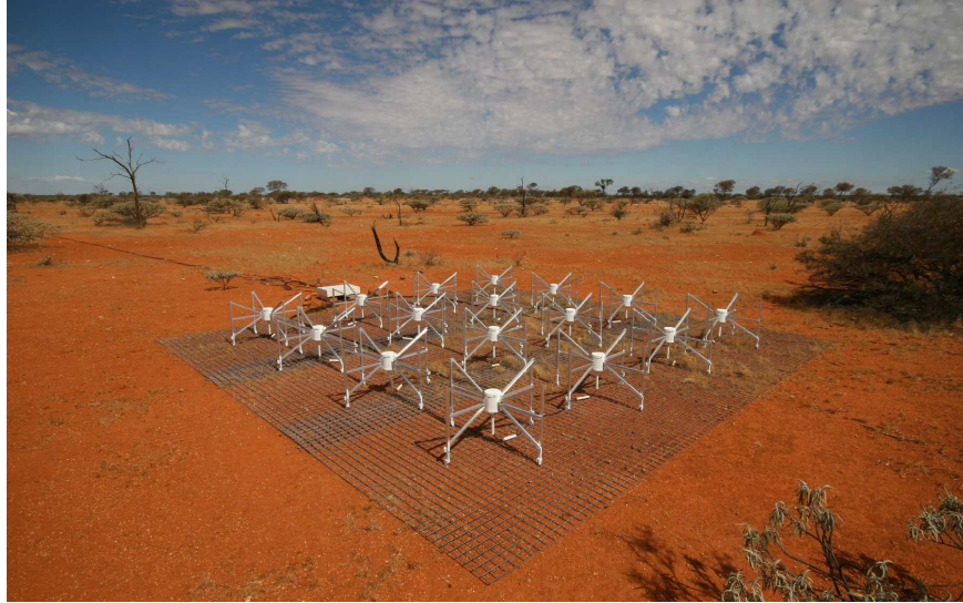
Figure 11.17 One of the antenna “tiles” used in the Murchison Widefield Array (MWA) experiment in Western Australia. Each such tile is composed of 16 crossed-dipole antennae, with their signals combined through hardware at the station. The full telescope combines the signals from \sim 128 tiles interferometrically. This allows for a large (several hundred square degree) field of view with a moderately large collecting area. The antennae operate between 80–300 MHz, corresponding to z \approx 6 –15 (although the telescope will only be sensitive to the spin-flip background at z < 10 ). Image credit: C. Lonsdale.
