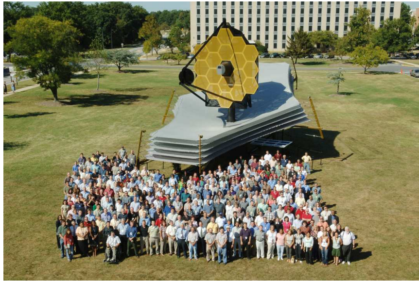
Figure 9.2 A full scale model of the James Webb Space Telescope (JWST), the successor to the Hubble Space Telescope ( http://www.jwst.nasa.gov/ ). JWST includes a primary mirror 6.5 meters in diameter, and offers instrument sensitivity across the infrared wavelength range of 0.6\text{--}28\mu\text{m} which will allow detection of the first generations of galaxies. The size of the Sun shield (the large flat screen in the image) is 22 meters \times 10 meters (72 ft \times 29 ft). The telescope will orbit 1.5 million kilometers from Earth at the Lagrange L2 point. Figure credit: NASA/EPO.
