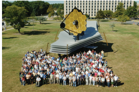
Plate 19 A full-scale model of the James Webb Space Telescope (JWST), the successor to the Hubble Space Telescope ( http://www.jwst.nasa.gov/ ; see Figure 10.2 and associated discussion for more information). JWST includes a primary mirror 6.5 m in diameter and offers instrument sensitivity across the IR wavelength range of 0.6 to 28 \mu\text{m} , which will allow detection of the first generations of galaxies. The size of the Sun shield (the large flat screen in the image) is 22 in \times 10 m (72 ft \times 29 ft). The telescope will orbit 1.5 million km from Earth at the Lagrange L2 point. NASA/EPO.
