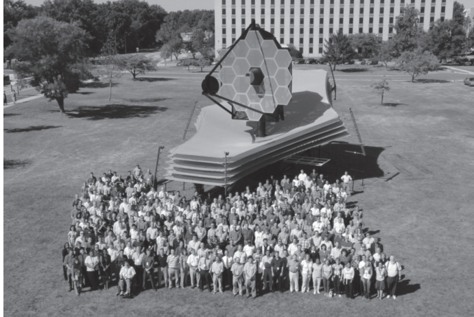
Figure 10.2 A full-scale model of the James Webb Space Telescope (JWST), the successor to the Hubble Space Telescope ( http://www.jwst.nasa.gov/ ; see Color Plate 19 for a color version of this image). JWST includes a primary mirror 6.5 m in diameter and offers instrument sensitivity across the IR wavelength range of 0.6 to 28\ \mu\text{m} , which will allow detection of the first generations of galaxies. The size of the Sun shield (the large flat screen in the image) is 22\ \text{m} \times 10\ \text{m} ( 72\ \text{ft} \times 29\ \text{ft} ). The telescope will orbit 1.5 million km from Earth at the Lagrange L2 point. NASA/EPO.
