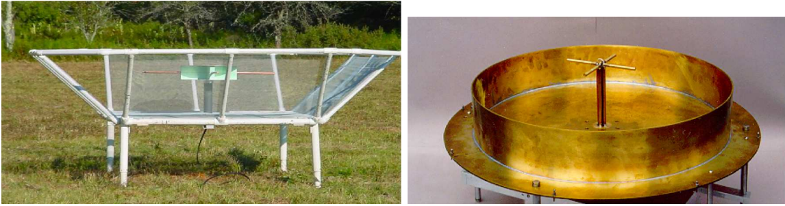
FIG. 18: Two examples of dipole-in-a-cavity antenna designs. Left : Prototype antenna from the PAPER experiment. Right : Antenna used in the STARE radio transient monitoring experiment.
