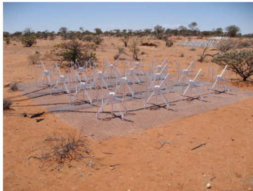
FIG. 15: Three MWA antenna tiles on site at the Radio Astronomy Park in Western Australia. These tiles are part of a 32-tile array that is currently under evaluation in preparation for construction of the full 512-tile array. Each tile consists of a four-by-four array of crossed dipoles operated as a phased array, an example of which can be seen in the foreground of this image.
