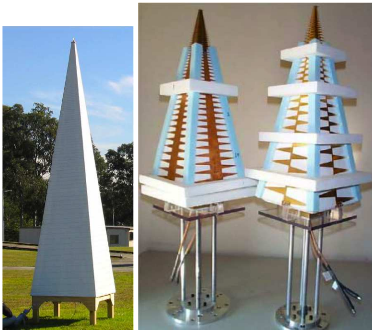
FIG. 19: Two examples of log-periodic antenna designs. Left : Prototype antenna from the CoRE experiment. Right : Prototype feeds for the Allen Telescope Array.
