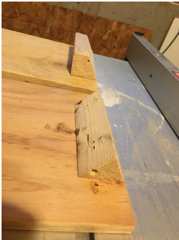
Figure 3. A couple of the blocks attached to panels. The bottom one is for one of the mirror mounts. The top panel shows the front-facing block that does not hold a mirror.
