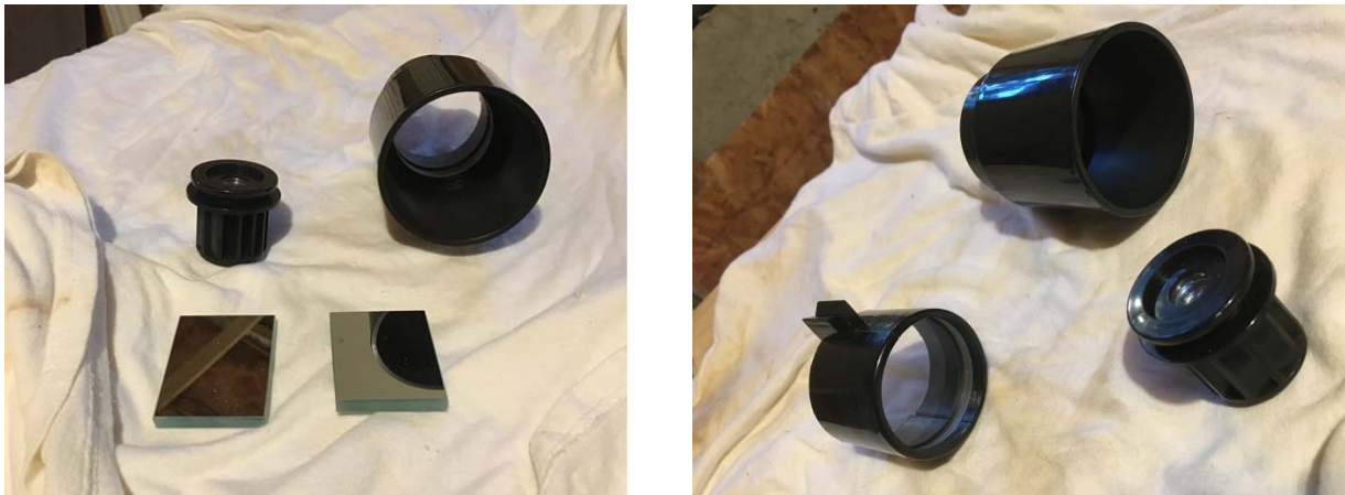
Figure 1. Optical components. The objective lens is from the Galileo telescope, the first-surface mirrors were purchased separately.
