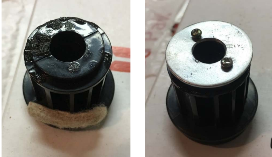
Figure 7. Effects of sunlight on the eyepiece. Left: The rear surface of the eyepiece showing heat damage. Right: The fix as implemented. A 1.25-inch washer with 0.5 inch center hole was attached to the back of the eyepiece.
