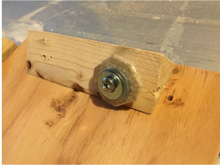
Figure 5. One of the screws with felt pad to hold the mirrors in place.
