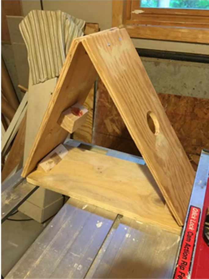
Figure 6. The final assembly before painting. A shim can be seen on the lower left corner wedge that was necessary to align the mirror.
