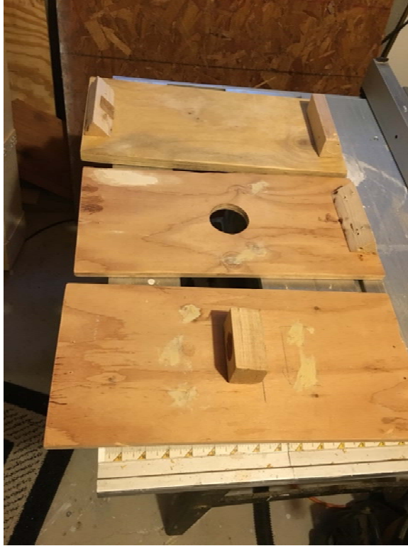
Figure 2. The three panels with blocks attached. The top is the base of the frame, the middle is the front-facing panel, and the bottom is the back panel with eyepiece holder.
