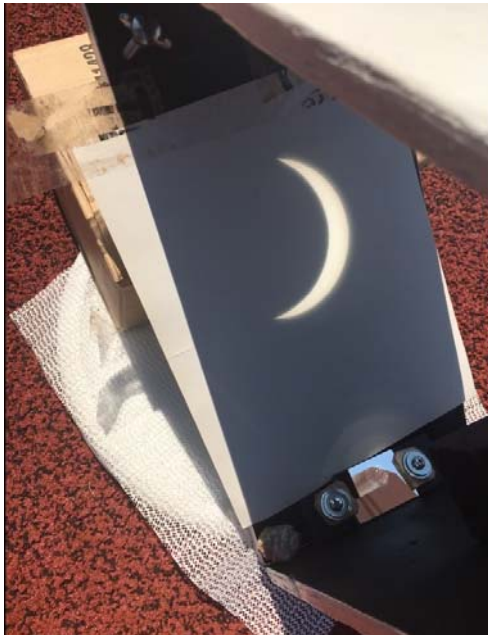
Figure 8. An image obtained during the August 21, 2017 eclipse, looking down from outside the front of the frame (visible in the upper right of the image). A white card is used to display the image projected by the optics. For the eclipse, a lazy susan was used to track the sun in azimuth. We did not have the cradle mount, so a box was used to adjust the altitude of the scope to track the sun.
