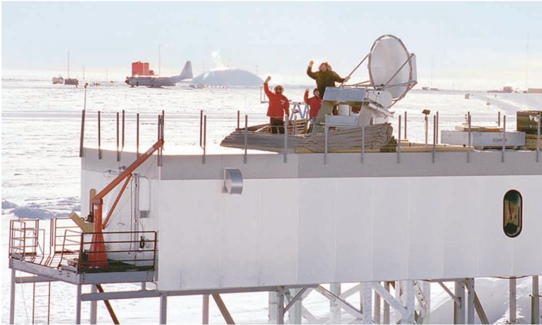
FIG. 1.—The Antarctic Submillimeter Telescope and Remote Observatory atop its building at the South Pole in 1997 February. Standing next to the telescope are G. Wright of Bell Labs and X. Zhang and A. Stark of Smithsonian Astrophysical Observatory. The telescope rests on a steel support tower which is structurally isolated from the building and can be covered by a fold-off canopy made of canvas and aluminum tubing. The main part of the Amundsen-Scott South Pole Station lies beneath the dome, which is about 1 km distant. An LC130 cargo aircraft is parked on the skiway. The South Pole itself is slightly below and to the right of the tail of the airplane. (Photo credit: A. Lane.)
