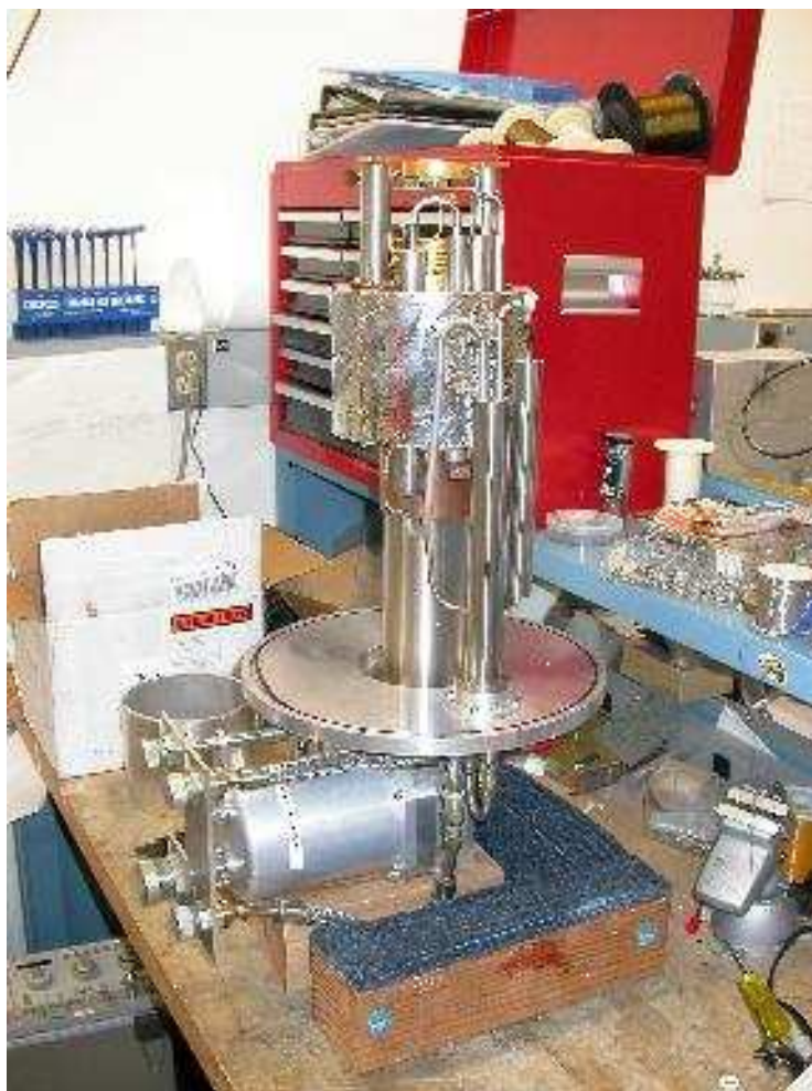
Figure 25: A photo of the DesertStar JT refrigerator. The small gold cylinder at the top of the refrigerator is the helium collection pot.
