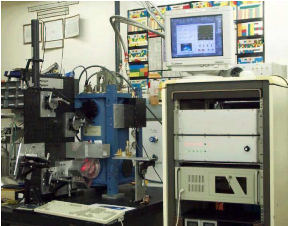
Figure 2: PoleStar in the lab during front-end testing. All system electronics fit into a single transportable equipment rack. A He-Ne laser is mounted on the optics plate here for optics alignment.
