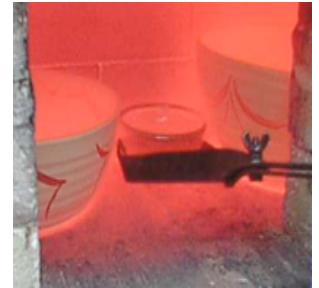
The pottery and brick walls in this kiln all glow with the same color.
