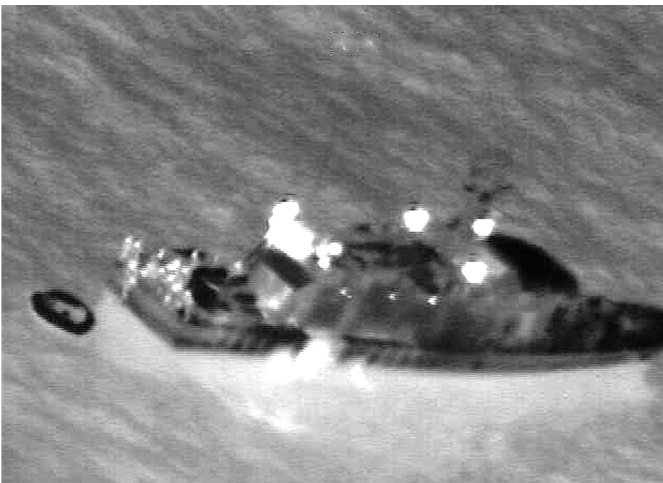
Figure 20: This is an image of a rescue vessel in the Red Sea taken from a US Navy patrol aircraft. The aircraft was using an infrared camera to search for survivors of a ferry accident. Notice that the people are bright white because they are warmer than the boat and water.
