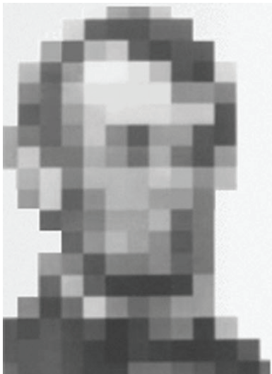
Figure 8: A digital image (left) is made of tiny squares or dots. The brightness of each square is represented by a number in the imagefile (right) that is stored in the computer. This image is made from only 8 shades of gray: the numbers run from 1 (black) to 8 (white). The numbers for only a few pixels are shown. Your eye can distinguish about 256 shades of gray — compared to 4096 for the MicroObservatory telescope!
