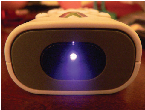
Figure 17: Although you can’t see it with your eyes, your television remote emits infrared light. Credit: Ed Poor http://en.wikipedia.org/wiki/File:Blue_infrared_light.jpg
