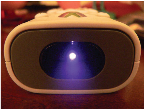
Figure 17: Although you can’t see it with your eyes, your television remote emits infrared light. Credit: Ed Poor http://en.wikipedia.org/wiki/File:Blue_infrared_light.jpg
