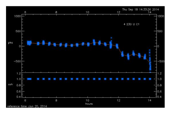
Select the frame that has the phase jump. Click/roll the middle button on your mouse to bring up the list of keyboard options. Type "w". This will select the option to phase-wrap.
