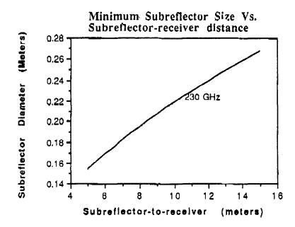
The subreflector 0.46 meter diameter subreflector used for the "baseline" calculation in Padman's report should be adequate for a flat-Nasmyth system, although you may want to increase the size further to reduce the required receiver aperture, as discussed in the next section. For a long Coude made entirely of flat mirrors a larger subreflector will probably be necessary.
