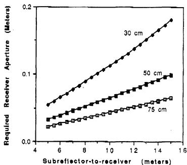
It should be noted that the "required receiver aperture" does not necessarily mean that the grids have to have a clear aperture as large as shown. Additional optics could be used at the receiver to cut down the beam size. An offset pair could be designed either for low cross-polarization or low illumination distortion, but probably not both.
