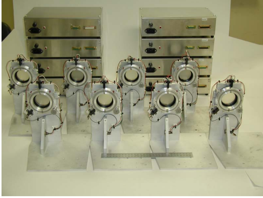
Fig. 1.— The SMA polarimetry hardware. The eight waveplates and positioning stages are in the foreground. These motor driven rotation stages allow rapid switching between LCP and RCP. Behind them are the eight control assemblies containing computers and power supplies.
