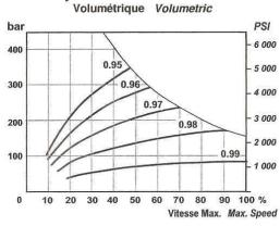
Mean values given as indication for displacement code 0, after 100 hours of use with HV46 hydraulic fluid @ 50°C [122°F].
