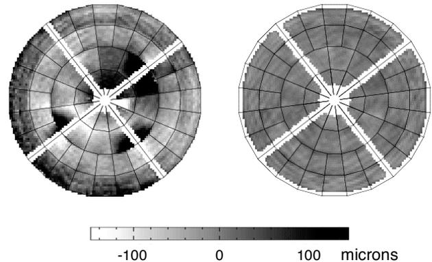
Fig. 3. The SMA antenna reflectors are typically set to 60  $\mu\text{m}$  rms (left) using a mechanical swing arm. A near-field holographic technique, using a phase-locked beacon at 232.4 GHz, is then used to progressively improve the surface. Three iterations are generally required to reach the design specification of 12  $\mu\text{m}$  rms (right).
