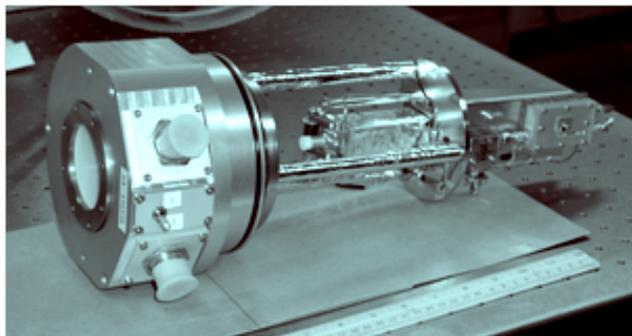
Fig. 5. Photograph of a 650 GHz receiver insert showing, from left to right, the vacuum window, electrical connectors, radial o-ring seal, interface to the 70 K radiation shield, mixer feed with Teflon dust cover. Further to the right: IF isolator and 4 – 6 GHz preamplifier.
