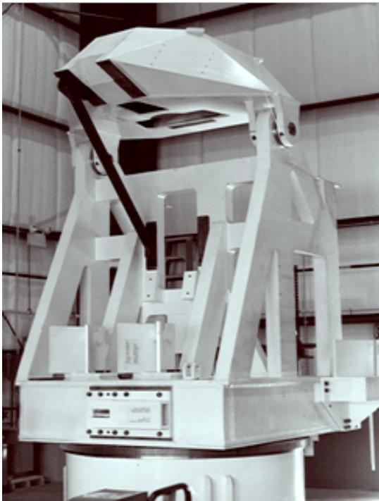
Fig. 2. Photograph of the SMA antenna pedestal. The structure above the elevation bearings connects to the reflector assembly.
