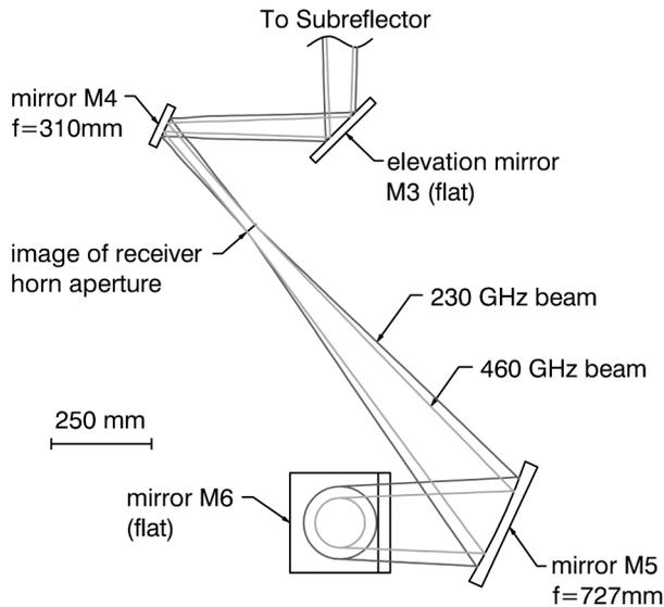
Fig. 4. The SMA antenna beam waveguide assembly used to couple radiation from the antenna to the receivers produces a compact image of the feed between the two ellipsoidal mirrors and provides a convenient location for receiver gain calibration and for the quarter wave plates required to enable polarimetry observations.
