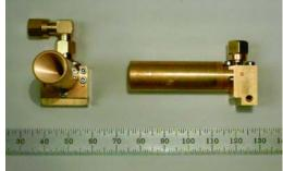
Figure 8: Left, photograph of a 650 GHz receiver insert showing, from left to right, the vacuum window, electrical connectors, radial o-ring seal, interface to 70 K radiation shield, mixer feed with Teflon dust cover, magnetic field coil, isolator and 4 – 6 GHz IF preamplifier. Right, photograph of a 345 GHz SIS mixer block.
