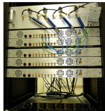
SWARM installation in laboratory, fed by sophisticated phase agile antenna simulator (J. Test poster)
