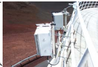
The 232.4/332 GHz and 692 GHz beacons on Subaru
