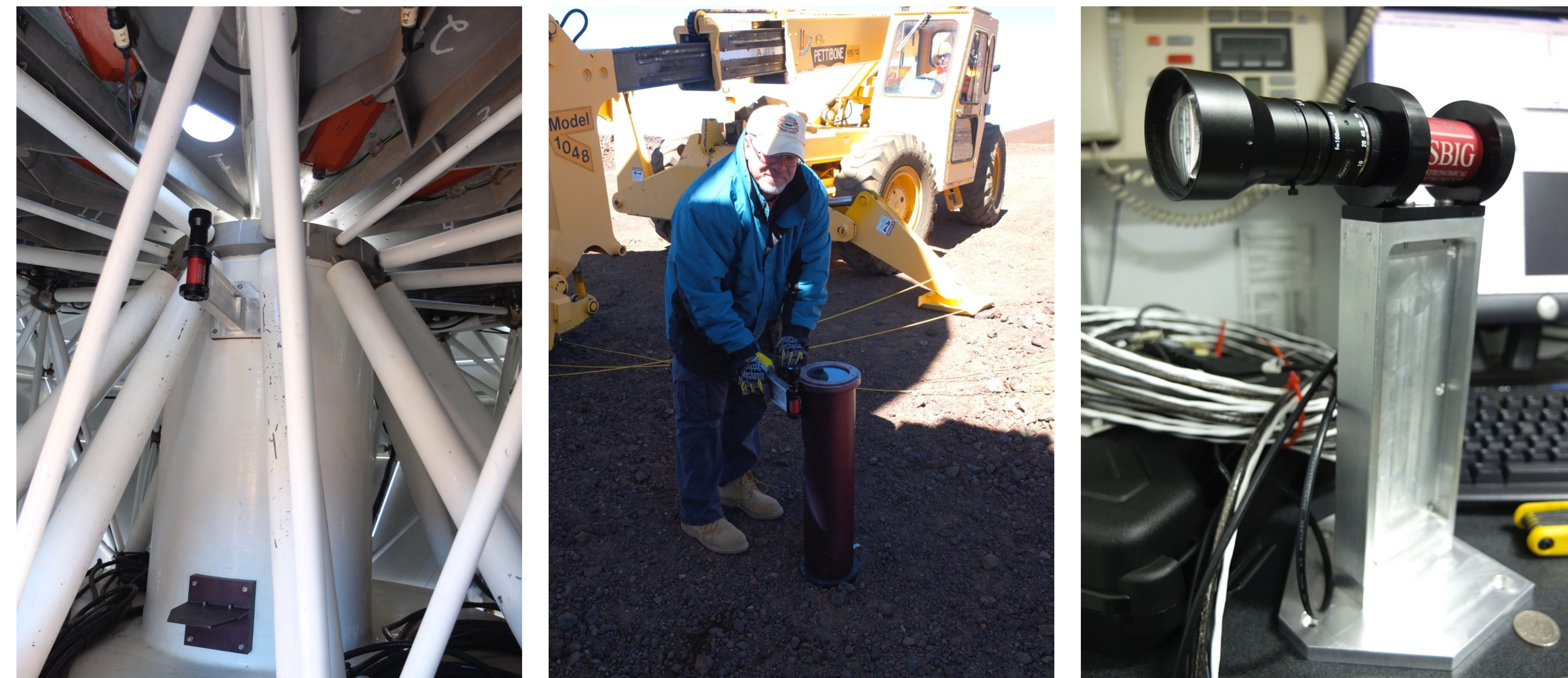
Figure 1: (Left) SBIG ST-i guide scope mounted on the carbon fiber central hub of the backup structure of SMA antenna-1. (Middle) Rob Christensen comparing the sizes of the old and new guide scope tubes! (Right): ST-i guide scope with the mounting bracket.
