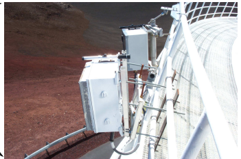
The 232.4/332 GHz and 692 GHz beacons on Subaru
