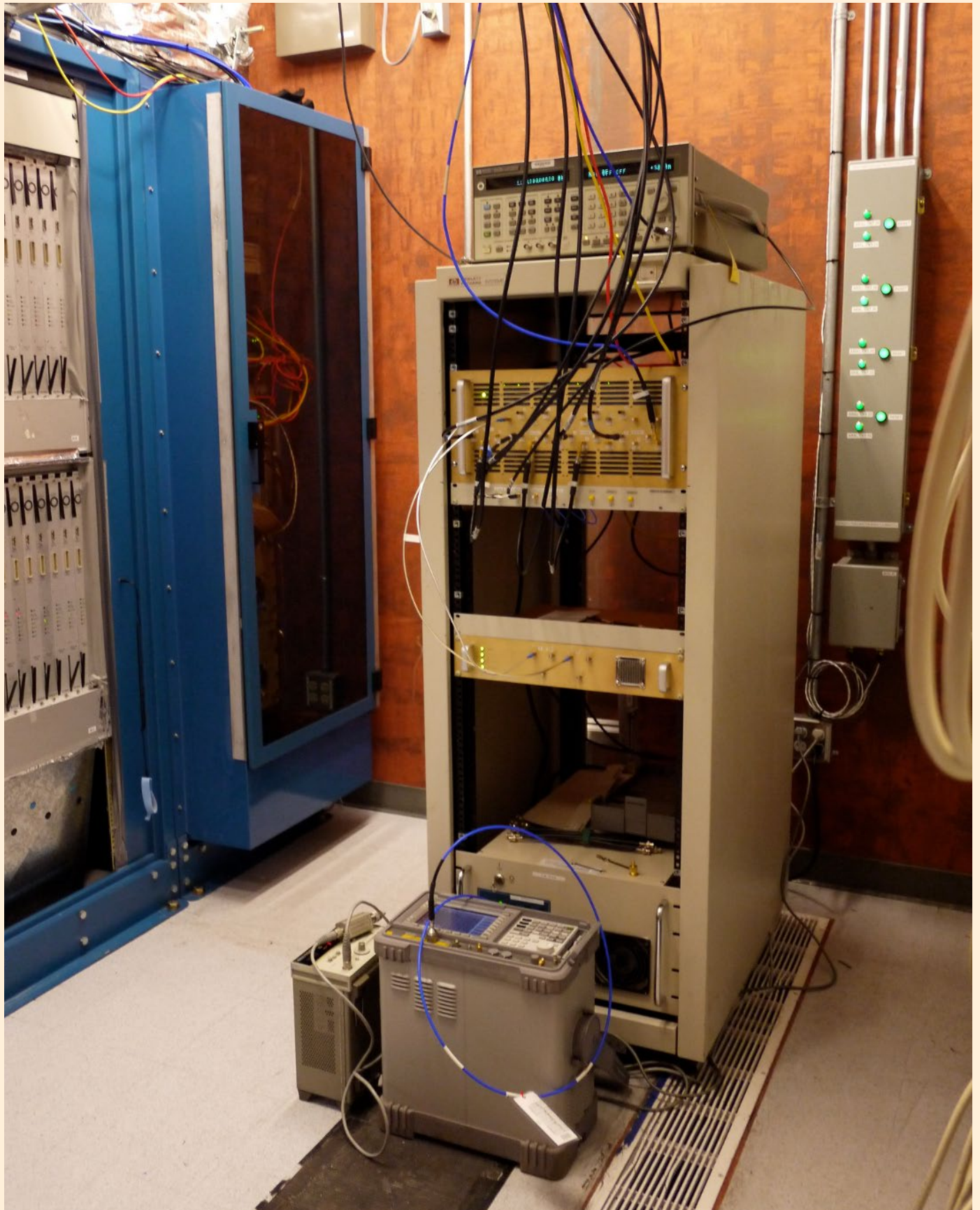
Figure 4: A photo of the DBE currently under development in the SMA summit correlator room. Photo courtesy of Derek Kubo.
