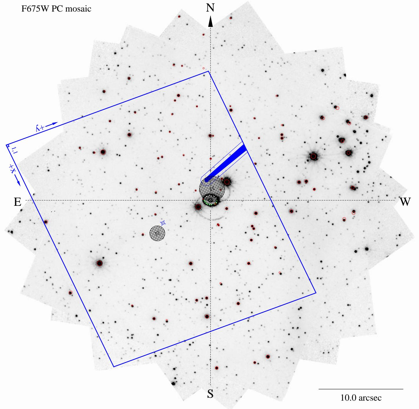
HRC Chip: 1024x1024 imaging area, as projected onto sky = blue parallelogram; pixel x=1,y=1 noted; center crosshair center crosshair = HRC-FIX aperture
