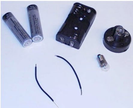
(Top left, clockwise) Batteries, case, socket, bulb, wires
