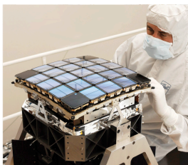
Focal Plane 95 Mega pixels, 42 CCDs
