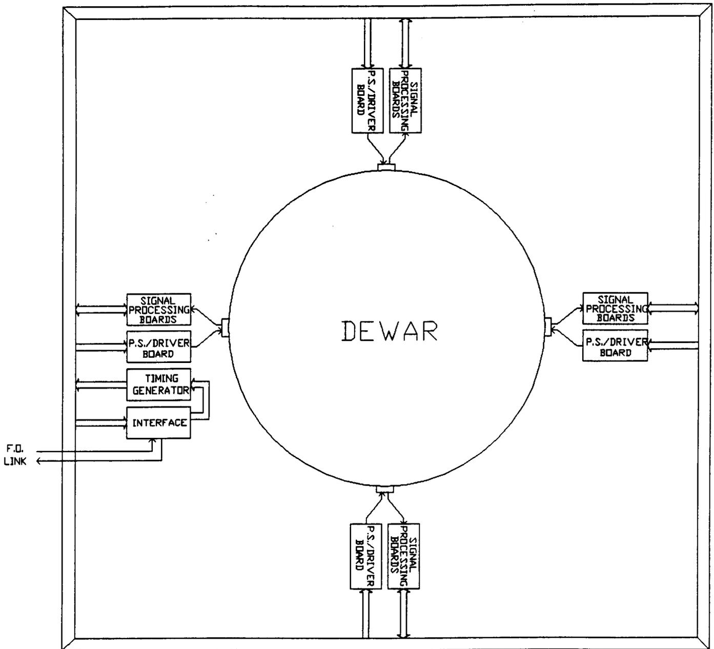
**Figure 1.** Physical partitioning of the S.A.O. Megacam. A single digital timing generator module transmits signals for CCD drive and signal processing to four ports around the circumference of the large dewar container, each handling up to nine 2K X 4.5K imagers (2 outputs each). Each signal processor board (four channels) will serialize its data and transmit to the camera interface, where the stream is demultiplexed and transmitted via fiber optic cable to the computer interface.
