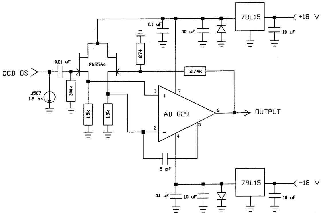
**Figure 3.** The fast-settling S.A.O. Megacam preamplifier design, utilizing the low-noise bipolar AD829 opamp with a 2N5564 dual JFET front end. Simple current feedback via the small 5 pf capacitor from inverting input to compensation pin proved effective in optimizing settling time.
