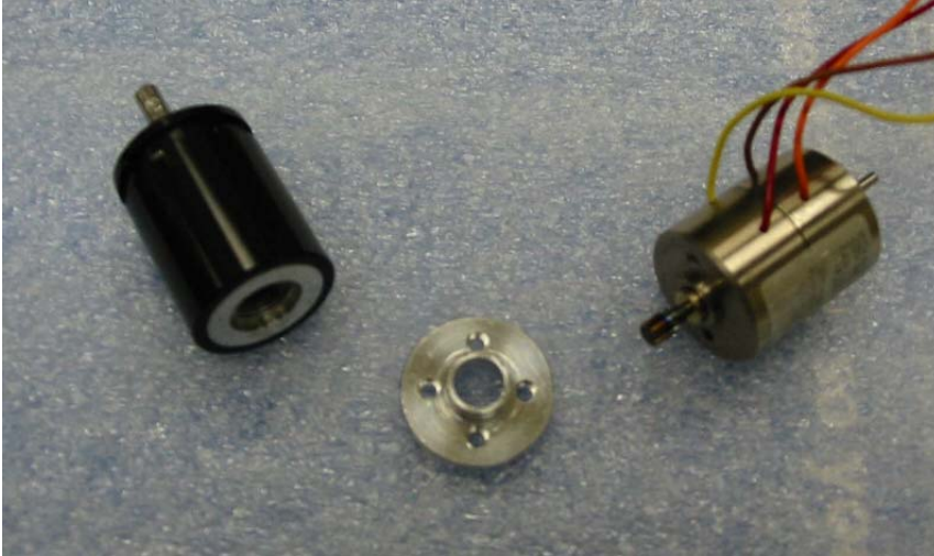
Figure 20. Gripper motor and gearbox disassembled.
