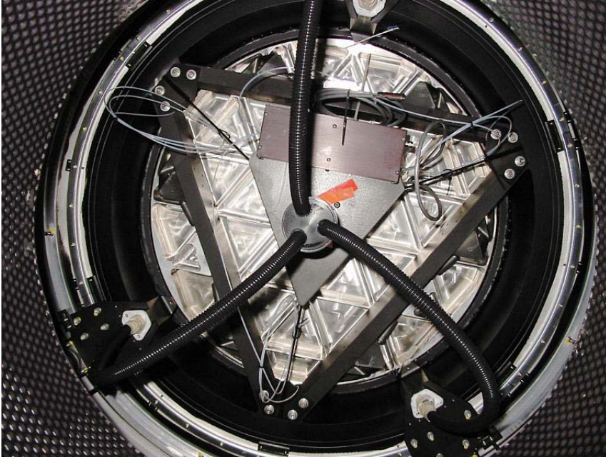
Figure 24. Photo of trifurcated coherent bundle and guide probes from beneath the focal surface.
