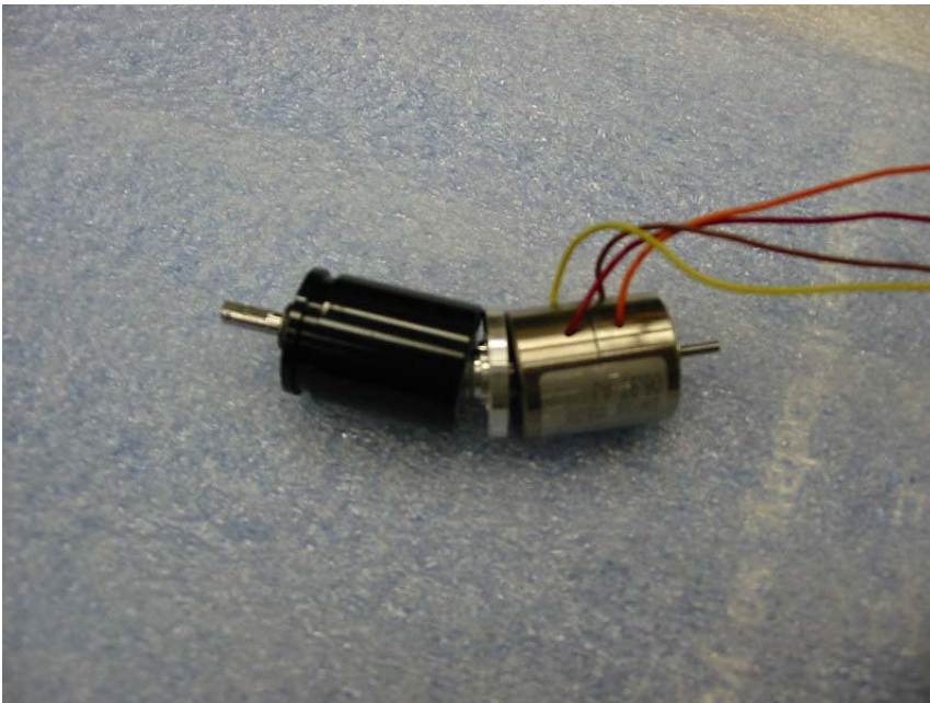
Figure 21. Gripper motor and gearbox partially assembled.
