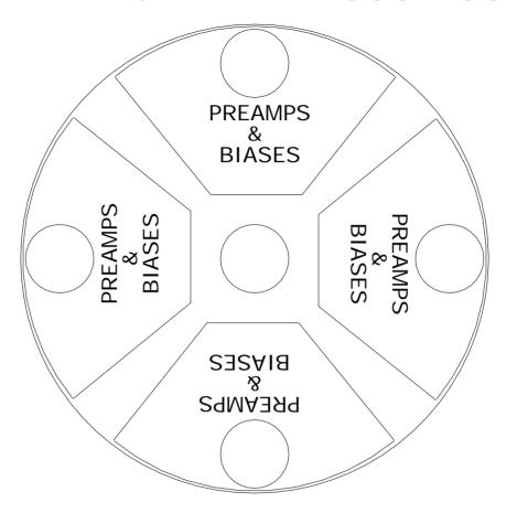
Each quadrant of the CCD will be serviced by one hermetic connector and associated cable down to the CCD dewar (18 pins each should suffice), with the preamp/bias printed circuits just outside the vacuum. A central connector is provided for thermal and shutter control, but we are unsure about the details of the latter control signal specification or whether it needs to enter at this point.
