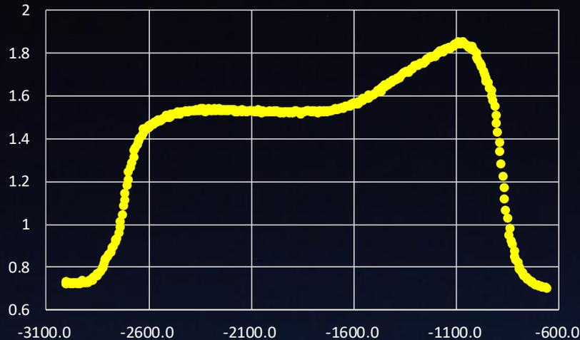
Azimuth scan of Moon with the GLT 86 GHz Receiver (observed frequency = 94.5 GHz) and with the Continuum Detector.
