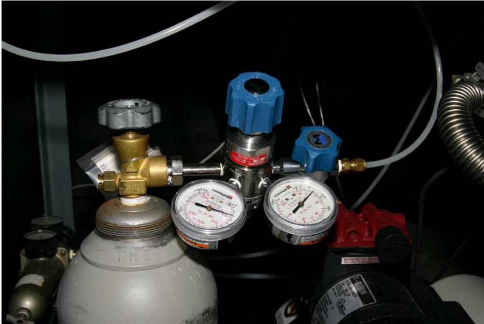
Figure 29. Back fill bottle. The middle blue valve is the pressure regulator control and normally should not be adjusted or turned. The backfill valves are the main bottle valve and the right hand blue valve.
