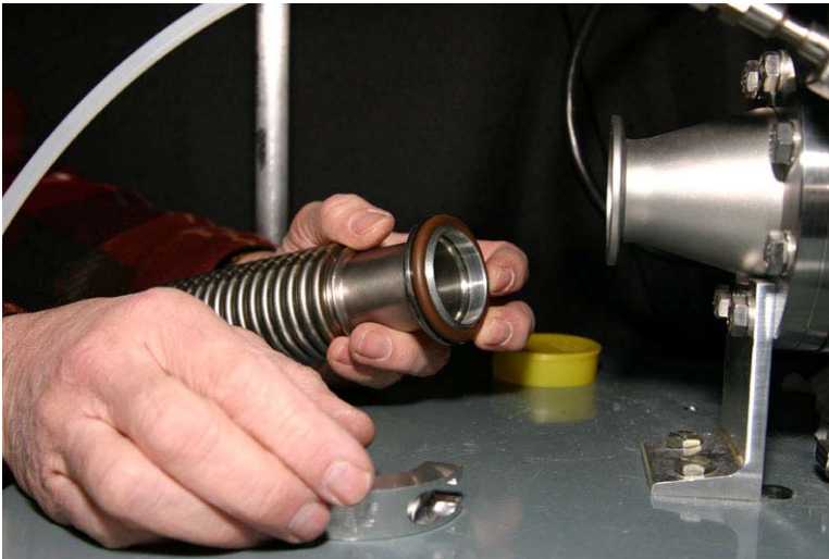
Figure 23. Pump station end of pump-out line.
