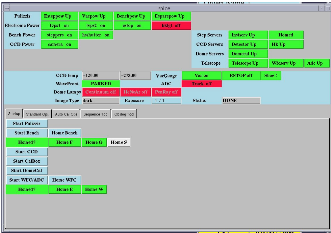
Figure 8. Spice Startup page. Use this to initialize software and home the three spectrograph motors. After this process is complete, return to the startup page for observing.
