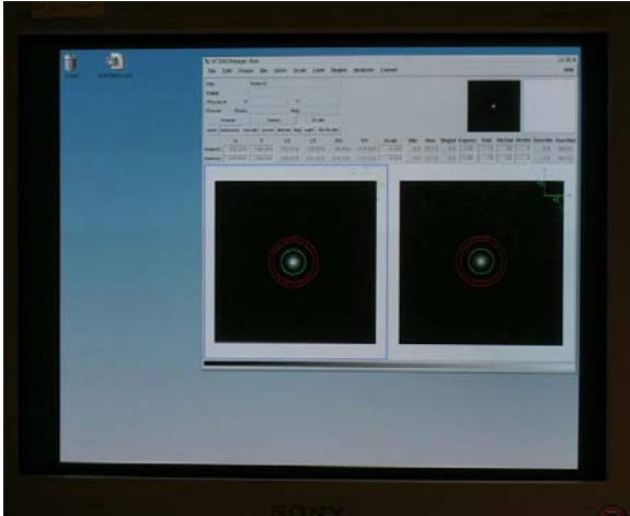
Figure 46. Robot camera display on second (rightmost) Fiber monitor. This display comes up after the Images button on the Hecto display is pressed.
